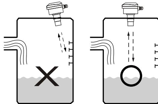
Mount the transducer away from the inlet to avoid interfere by medium.
