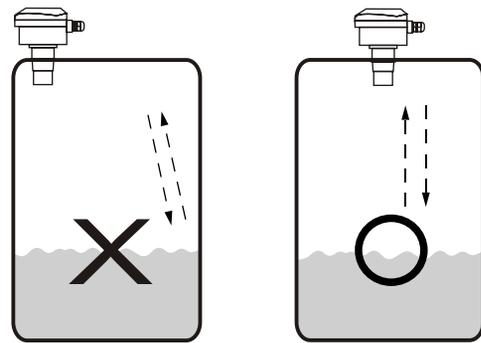
A pipe surrounding the detection path along the ultrasonic wave from emitting to receiving is recommended, thus installation can prevent fake signal caused by turbulence and foam when agitator is equipped in the tank. When the pipe is installed, a vent hole is required to balance the pressure difference between the inside and outside of pipe.
