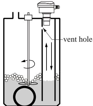
Do not mount the device close to the tank wall in case the fake signal caused by the bracket.
