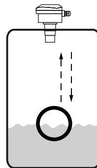
A pipe surrounding the detection path along the ultrasonic wave from emitting to receiving is recommended, thus installation can prevent fake signal caused by turbulence and foam when agitator is equipped in the tank. When the pipe is installed, a vent hole is required to balance the pressure difference between the inside and outside of pipe..
