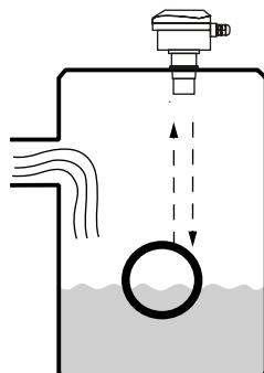
When user mount the transducer on the solid tank, the transducer must point to the outlet of tank.
