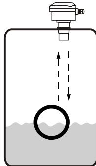
The transducer should not be mounted too close to the tank wall to avoid interference caused by the tank wall.
