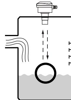
Mount the transducer away from the inlet to avoid interfere by medium.
