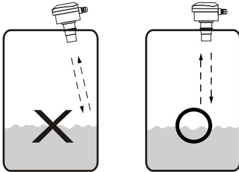
The transducer should not be mounted too close to the tank wall to avoid interference caused by the tank wall.
