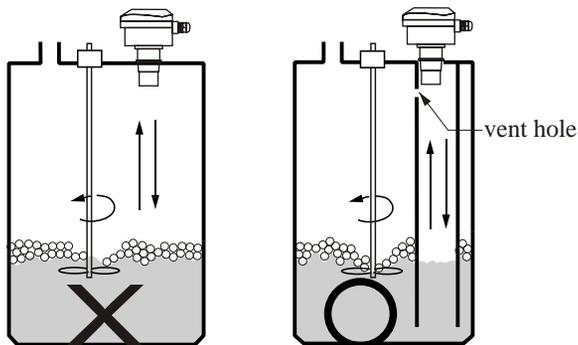
Do not mount the device close to the tank wall in case the fake signal caused by the bracket.
