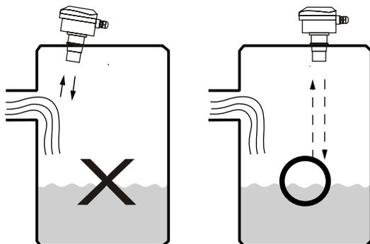
When user mount the transducer on the solid tank, the transducer must point to the outlet of tank.
